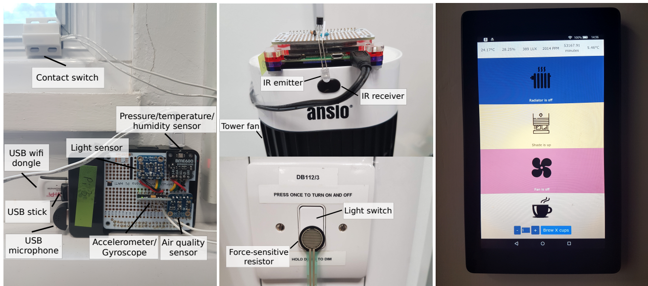
(a) The sensor configuration for one of the Raspberry Pis. A detailed listing of the sensor configuration can be found in Table 3. The contact switch at the top is being used to detect when the window is being opened or closed.
