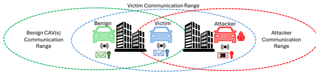
Figure 3: Illustration of the hidden terminal scenario.
