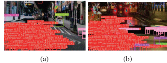
Figure 13: Phantom Sponge “universal” perturbations created on primarily dark-colored data will only affect dark surfaces.
